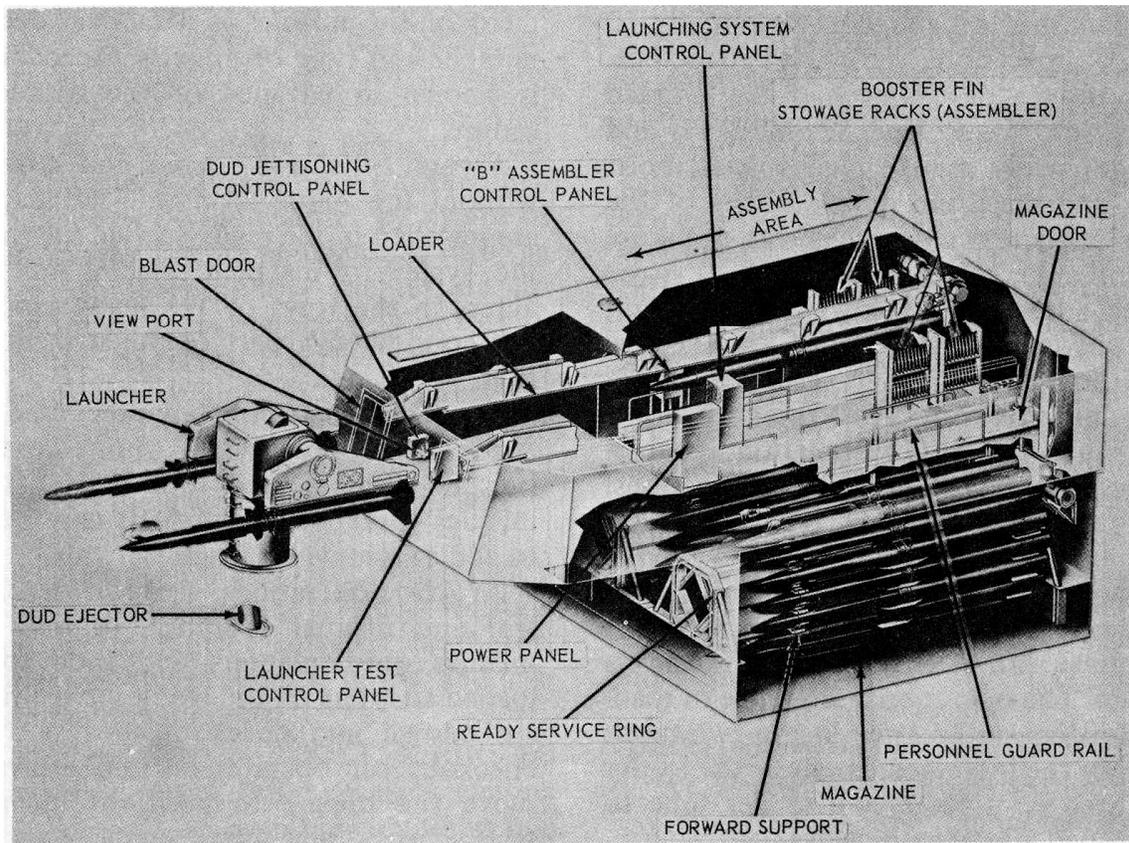
Figure 2-8.—Guided missile launching system Mk 10 Mod 0.
